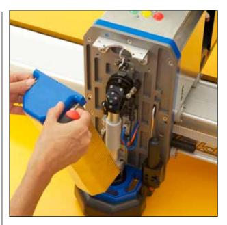
The Elektron Laser ZT is designed for easy maintenance with major components easily accessible.
