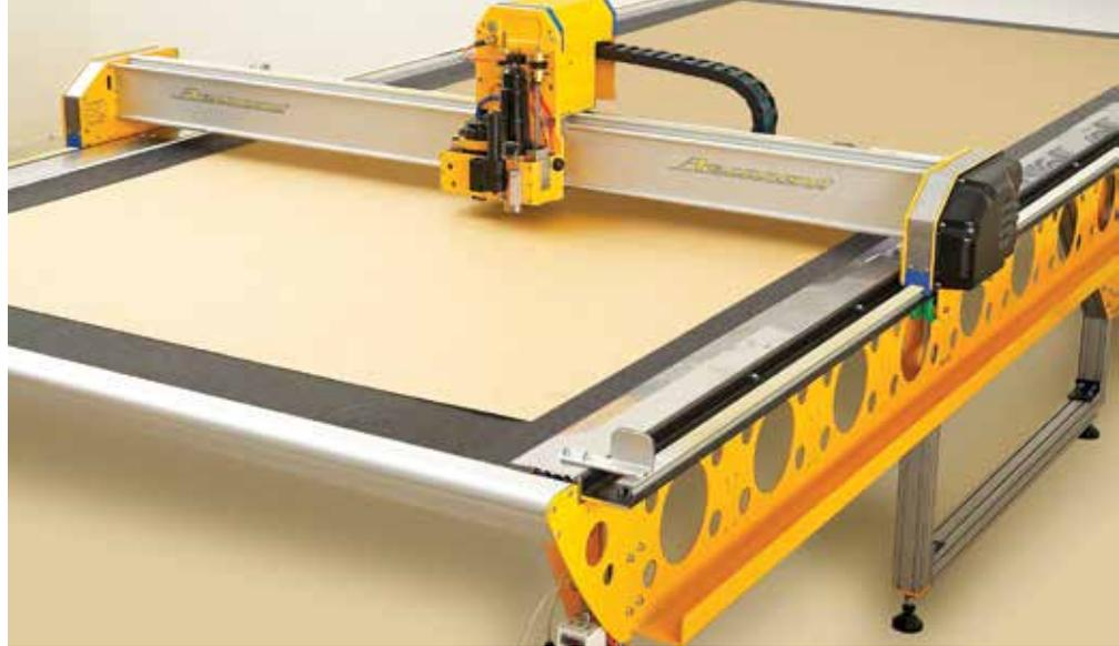
Because Aeronaut operates in several markets in the industrial and technical textiles field, cutting tables can be as small as 1200mm x 1200mm or as large as 10 metres by 50 metres and longer. These giant machines are used for tasks as varied as making high tech yacht sails to drawing paint-by-numbers markings on carpet backing for manufacturing hand made carpets.
